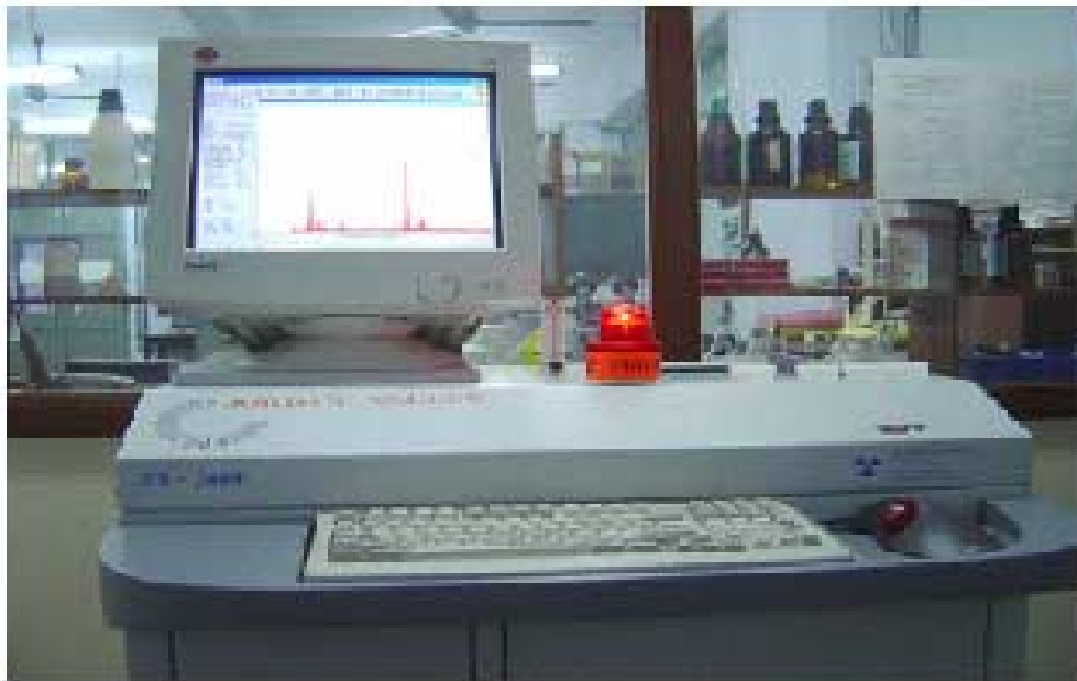
Energy Dispersive X-ray Fluorescence Set-up for Trace Element Studies at UGC-DAE CSR, Kolkata Centre.
