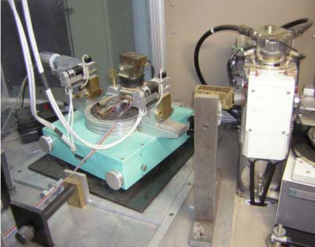
X-ray reflectivity and X-ray standing wave setup developed inhouse at CSR, Indore Centre.
