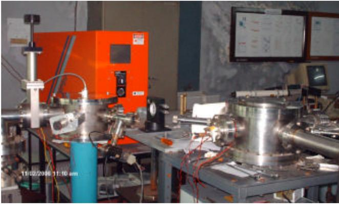
Fig. 1: Photograph of pulsed laser deposition system at UGC-DAE CSR, Indore.
