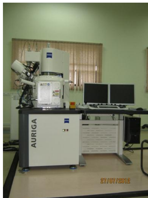
Photograph of FIB-SEM AURIGA instrument from M/S Carl Zeiss, Germany.
