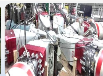
CLOVER DETECTOR SETUP AT VECC
