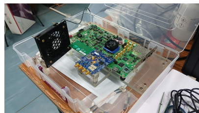
Figure 2: FPGA board with compatible ADC card and cooling system at Kolkata Centre.
